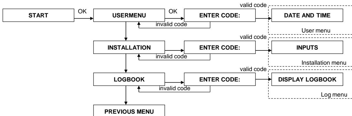
The user menu is only accessible with the supervisor code (code number 90, default code = **445566**). From software V2.03 and above also 4-digit codes can be used. Use this code once to enter the user menu and change the supervisor code immediately.
